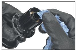
3. Grease both bearings and the inner side of both end caps.
