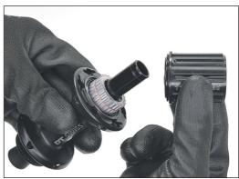
3. Remove springs, ratchets and spacer from the hub.
