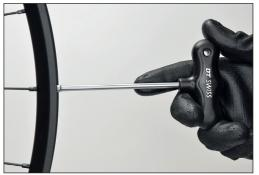
With the help of the DT Swiss nipple key, the nipple can be turned on the outside of the rim. This is the common method for:
