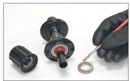
3. Fit the ratchet, the spacer and the spring.
