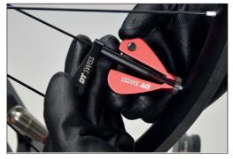
Flat spokes must be held while the nipple is tightened and loosened. This must be done with a spoke holder depending on the spoke type. It is important here to ensure that the spoke holder is pushed as far as possible in the direction of the nipple.
