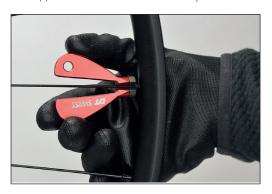
With the help of the DT Swiss Spokey, the nipple can be turned on the inside of the rim. This method is particularly useful for:
