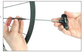
3. Also completely unscrew the nipple of the spoke that crosses the spoke to be changed at the hub flange.
