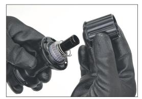
3. Grease the bearings and the inner surface of both end caps.
