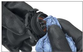
3. Grease the bearings and the inner surface of both end caps.
