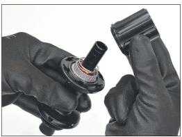
3. Remove the spring, the ratchet and the spacer from the hub.
