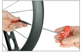
3. Also turn out completely the nipple of the spoke that crosses the spoke to be changed at the hub flange.
