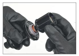
3. Grease both bearings and the inner side of both end caps.
